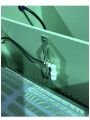
The top sensor can only be adjusted correctly when the system is commissioned.
